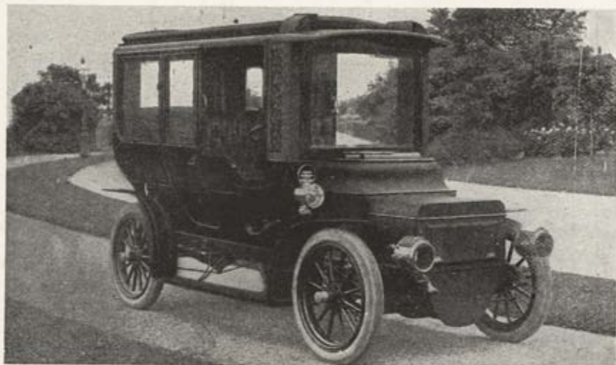
The Johnson Steam "Auto-Carriage," 30 H. P., single acting steam motor placed forward; bore 3\frac{1}{2} in., stroke 4 in., semi-flash boiler 20 \times 20 \times 17 in., burner 20 \times 20 in., tread 56 in., wheel base 108 in., wheels 38 \times 4 in., weight 3250 pounds; passenger capacity 5 to 7; price $3500, with all accessories.
